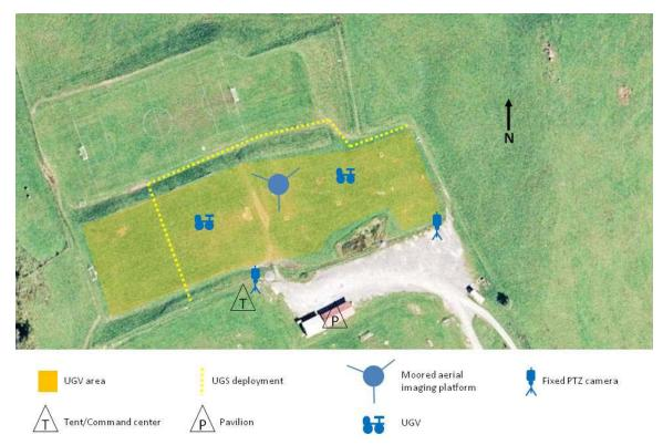
Figure 12. Overhead view of soccer field and placement of sensors
