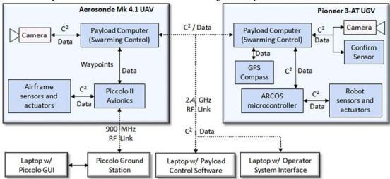
Figure 4. UAV and UGV System Architecture for Surveillance Demonstration
