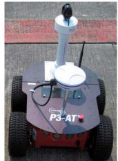
Figure 2. Pioneer 3-AT ground robot
