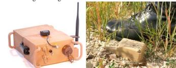
Figure 10. Crane MicroObserver gateway and 1045 acoustic and seismic sensor
