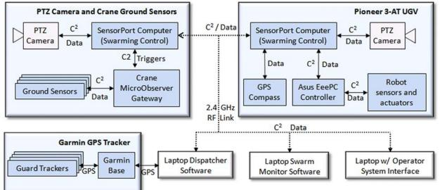
Figure 11. UGV, Ground Sensor, PTZ Camera Architecture for Perimeter Protection Demonstration
