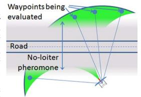
Figure 7. No-Loiter Pheromone minimizes time UAV spends overflying highway
