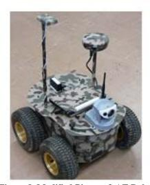
Figure 8. Modified Pioneer 3-AT Robot for Facility Patrol
